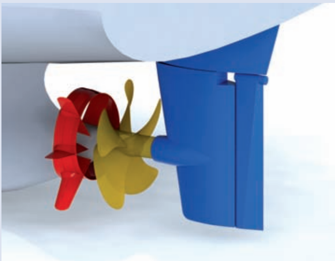
Becker twisted Fin® and bulb rudder arrangement
