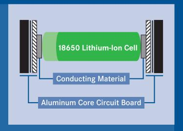
energy standard cells. Elastic cell bonding provides a secure contact for the entire service life as well as maximum resistance to vibration. Employing standard, high-quality 18650 cells with high energy density, COBRA is able to generate outstanding performance by interconnecting a high number of cells using only a few robust assembly components and connectors.
