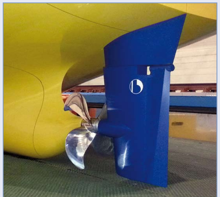
Cross Over Rudder model for performance test at Korean model test facility.
