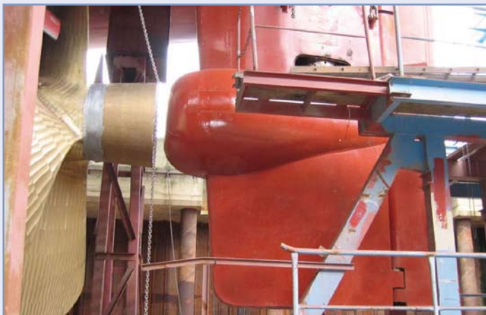
Cross Over Rudder for single screw feeder vessel Cape Flores, 1,200 TEU.
