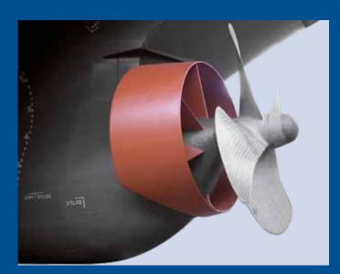
propulsive power. Both effects contribute to one another. The power savings attainable from the Becker Mewis Duct® are strongly dependent on propeller thrust loading, from 3 to 8% depending on individual hull/propeller interaction. The power savings are virtually independent of ship speed. The Becker Mewis Duct® is ideally suited to both new-build and retrofit applications (e.g. tankers, bulkers and MPCs).
