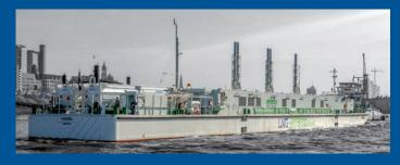
Becker's LNG Hybrid Barge generates energy for cruise ships lying at port. Compared to the current method of producing energy using onboard diesel engines, power supplied by the LNG Hybrid Barge will lead to a dramatic reduction of harmful CO<sub>2</sub>, NO<sub>x</sub>, SO<sub>x</sub> and particle emissions during layovers at port.
