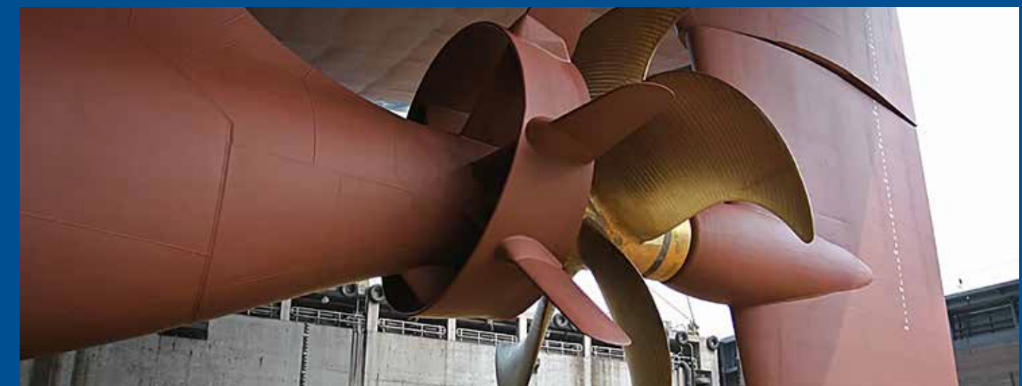
The Becker Performance Package: A Becker Rudder in combination with a Becker Mewis Duct® or Becker Mewis Duct® Twisted
